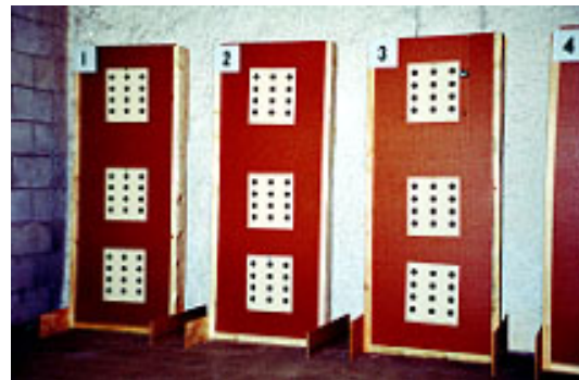
10-meter air rifle range target holders with targets placed at the proper heights for firing from the prone, kneeling, and standing positions.
